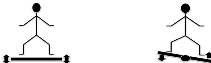
**Figure 1(a):** Vertical vibration platform      **Figure 1(b):** Side-alternating vibration platform
